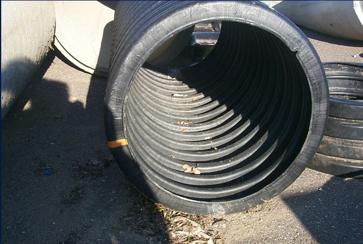
**Add a comment because single wall corrugated HDPE should not be used as highway culverts or storm drain.**
